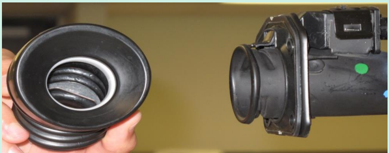
Boot overlaps fill pipe
