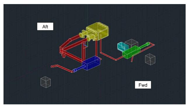
Figure 8. Dredge Thruster and Generator Engine Retrofit Arrangement with Point Cloud Suppressed
