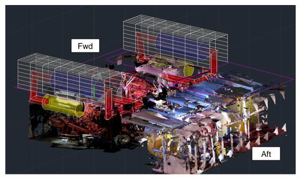
$\circ\,\mbox{The red represents the new exhaust piping path.}$
