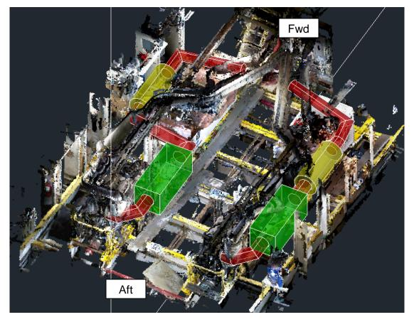
Figure 11. Excursion Vessel Retrofit Arrangement
