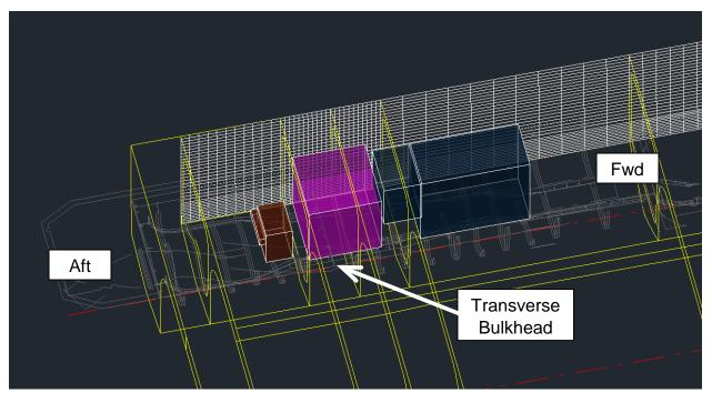
Figure 16. High Speed Ferry Repower Arrangement (Port Hull Shown)
