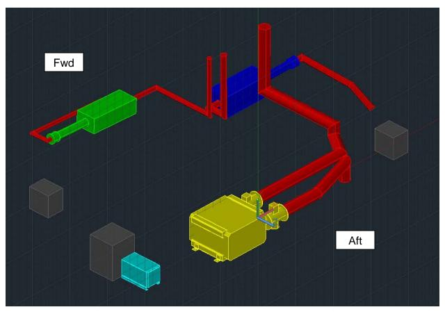
Figure 6. Dredge Pump/Winch Engine Repower Arrangement with Point Cloud Suppressed
