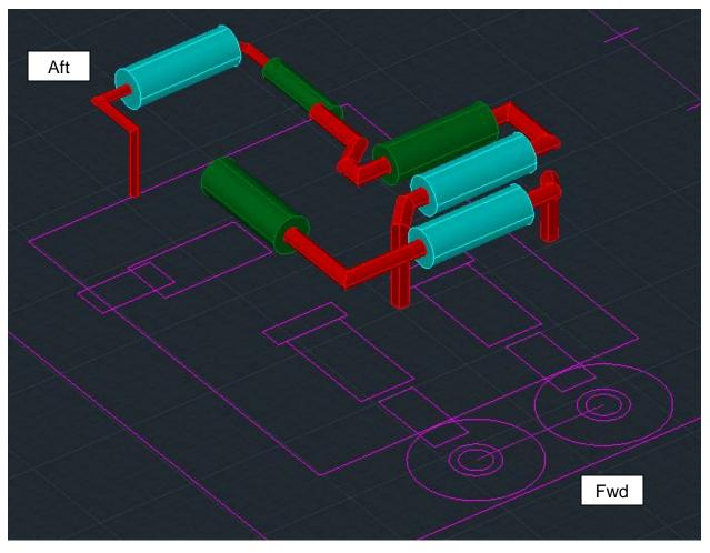
Figure 4. Barge Stbd Engine Room Retrofit Arrangement with Point Cloud Suppressed
