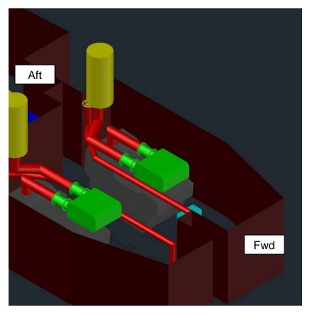
Figure 18. Ship Assist Tug Repower Arrangement
