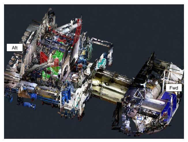
Figure 19. Push Tug Repower Arrangement
