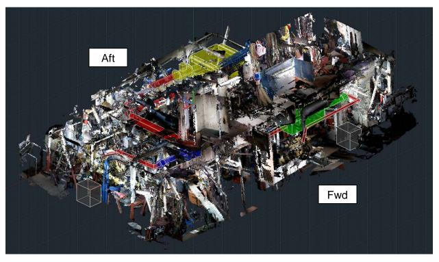
Figure 7. Dredge Thruster and Generator Engine Retrofit Arrangement
