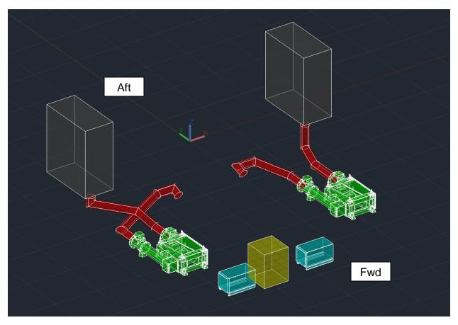
Figure 15. Slow Speed Ferry Repower Arrangement with Point Cloud Suppressed
