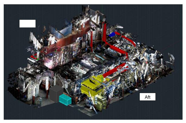
Figure 5. Dredge Pump/Winch Engine Repower Arrangement
