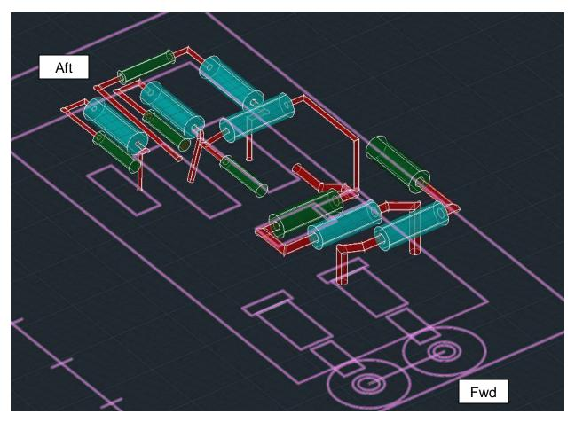
Figure 2. Barge Port Engine Room Retrofit Arrangement with Point Cloud Suppressed
