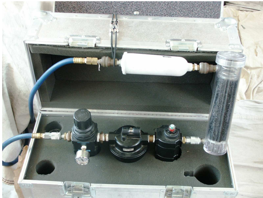
Figure A-0-2 Field Processing Unit for Purifying Dilution Air in Transport Case
