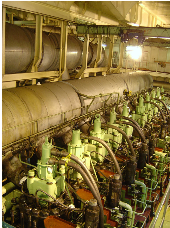
Figure 2-1 Picture of the Fuel Injectors on an Engine from the 11K90MC-C Series
