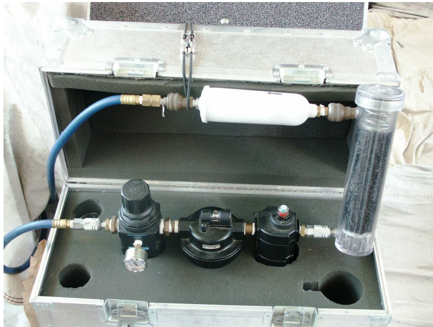
Figure 6-2 Field Processing Unit for Purifying Dilution Air in Carrying Case
