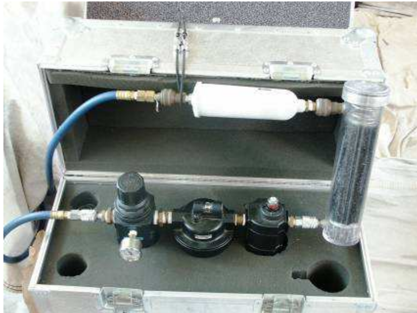
Figure 7-2 Field Processing Unit for Purifying Dilution Air in Carrying Case
