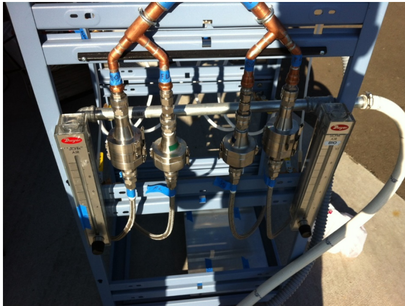
Figure II-3 Photograph of two stage filter system for soot and fuel burning phases.
