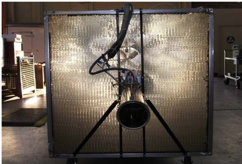
Figure II-2 – Honeycomb inlet section of small wind tunnel with connection pipe for the truck exhaust pipe.
