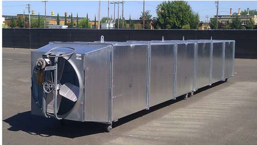
Figure II-1 – Small wind tunnel with attached whole house fan. Tunnel length is 30' and the cross-sectional area is 4' by 4'.
