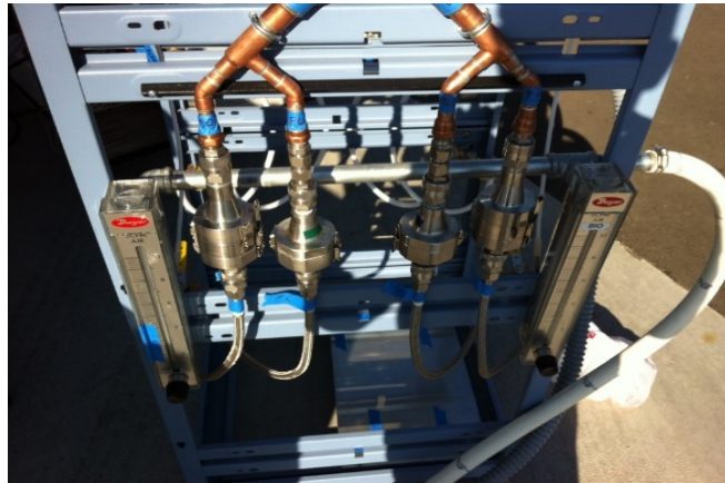
Figure ES-2 Photograph of two stage filter system for soot and fuel burning phases.
