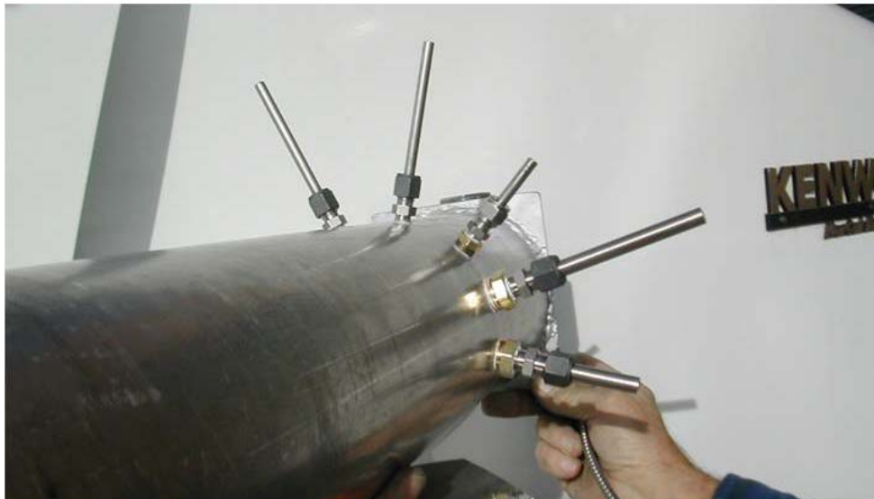
Figure II-4 Sampling tube with individual ports for emission instrumentation.
