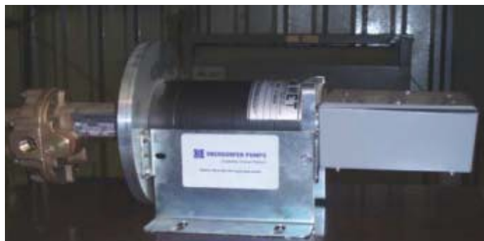
Solar-charged glycol pump (Source: BP)
