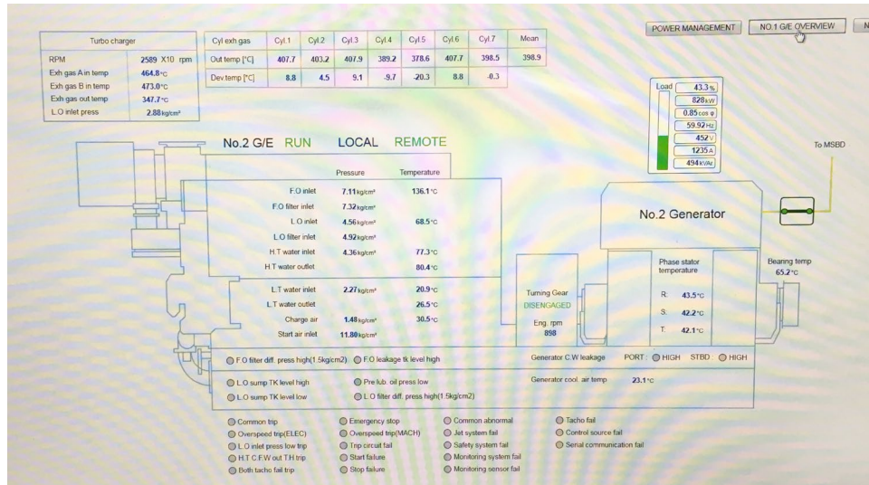
Figure D-4 Auxiliar diesel generator #2 loads and particulates (under test).
