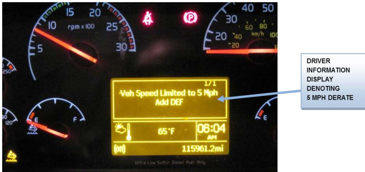
Figure Volvo-5: Volvo Driver Information Display Indicating 5 Mph Derate
