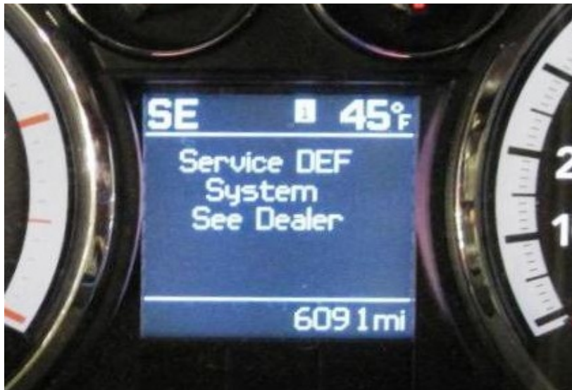
Figure Cummins 6.7-6: Tampering Message
