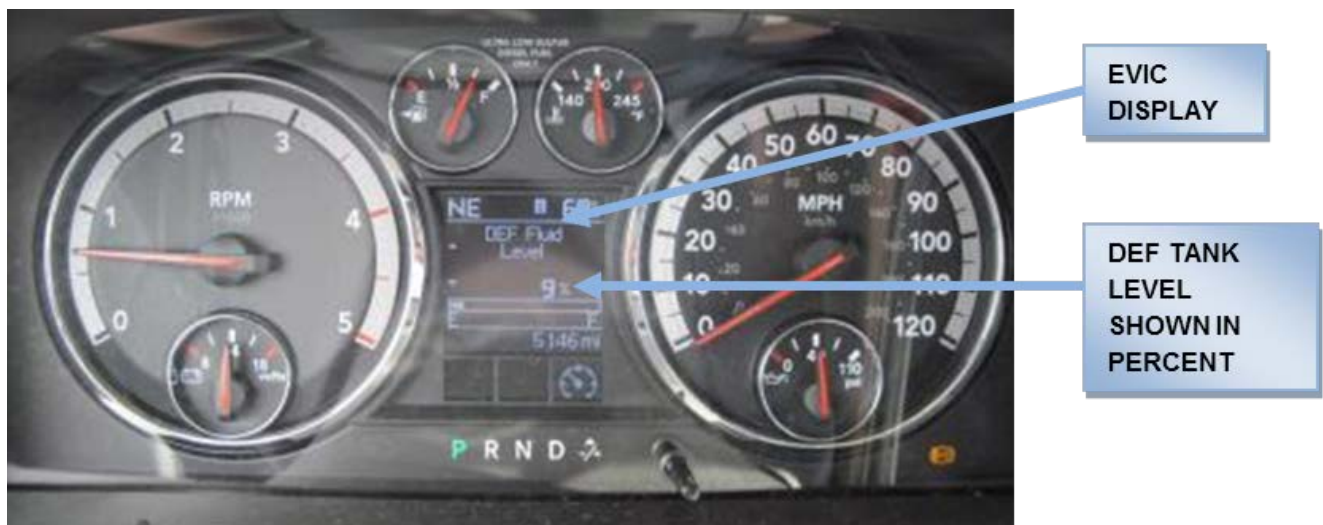
Figure Cummins 6.7-2: Electronic Vehicle Information Center
