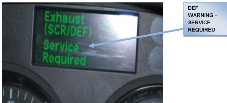
Figure Cummins 14.9-8: DIC Message – Exhaust (SCR/DEF) Service Required
