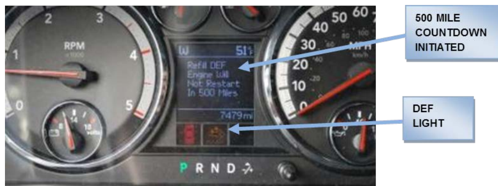
Figure Cummins 6.7- 4: Example of Message Alert, 500 Mile Countdown
