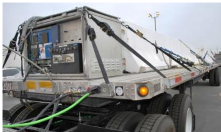
Figure DDC-2: Portable Emissions Monitoring System and K-Rails
