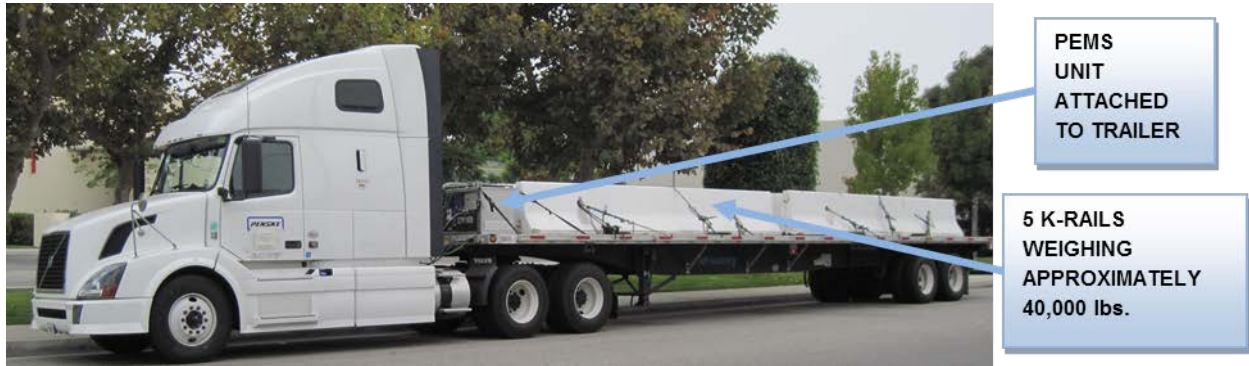
Figure Volvo-2: Portable Emissions Monitoring System and K-Rails
