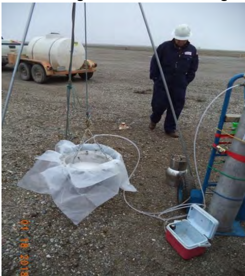
Photo Showing Flux Chamber Testing.
