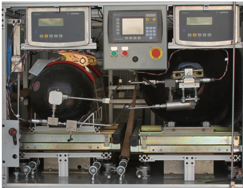
Figure 19: Hydrogen Field Standard Dispenser Accuracy Testing Device
