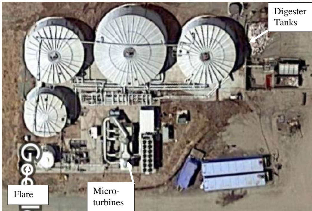
Figure 2-2: Over-view of READ biogas production facility.
