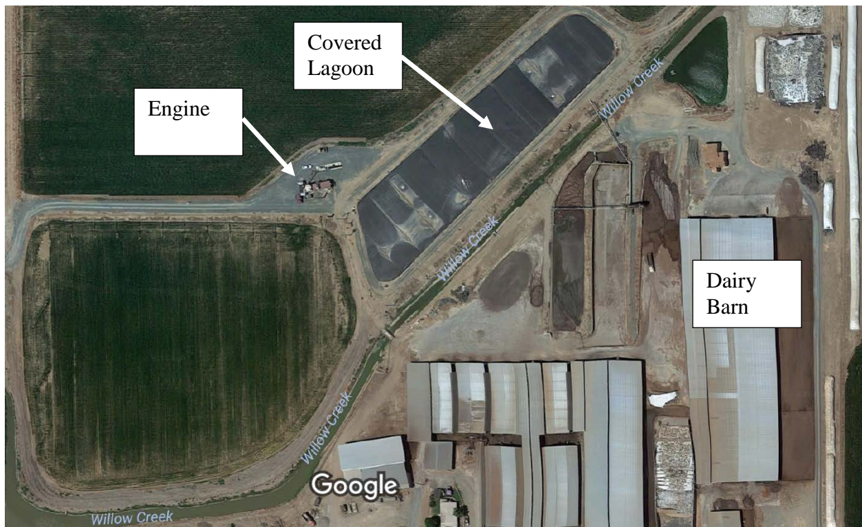
Figure 2-5: Over-view of VanWarmerdam dairy biogas production facility.
