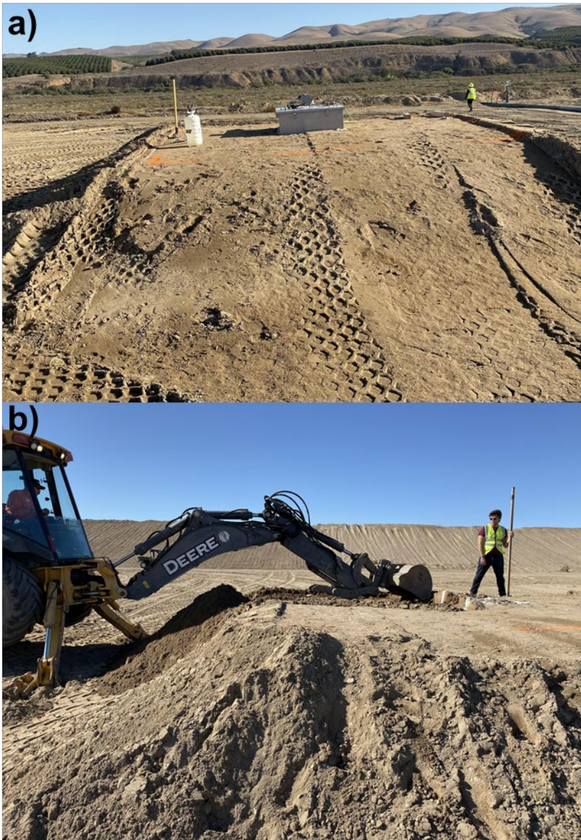
Figure 3.25 a) Static Flux Chamber Testing on the Test Plot Constructed at SMRL, b) Removal of 0.3 m-thick Soil Layer for Testing the Next Cover Thickness.
