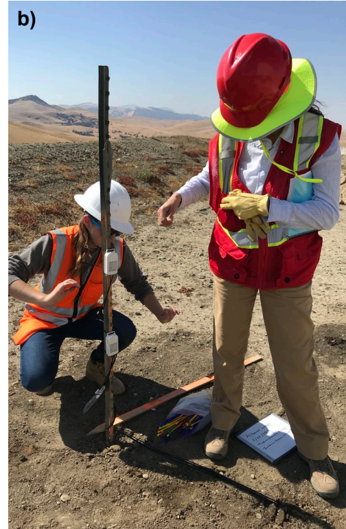
Figure 3.13 Installation of Thermocouple Array and Field Temperature Measurement
