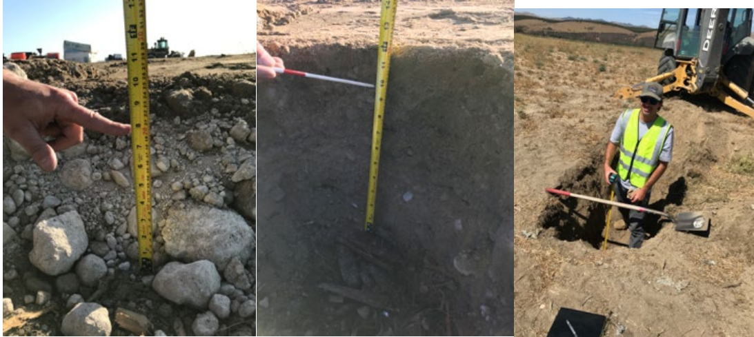
Figure 3.15 Cover Thickness Characterization
