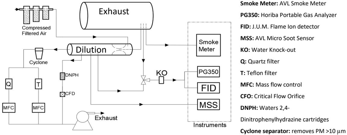
**FIGURE 5 SCHEMATIC SHOWING LAYOUT OF UCR EQUIPMENT**
