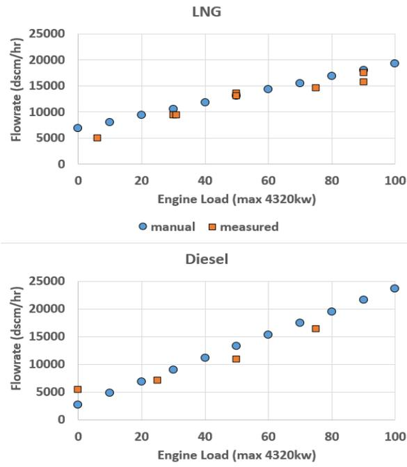
FIGURE 6 FLOW EXHAUST RATE IN DRY STANDARD CUBIC METER PER HOUR
