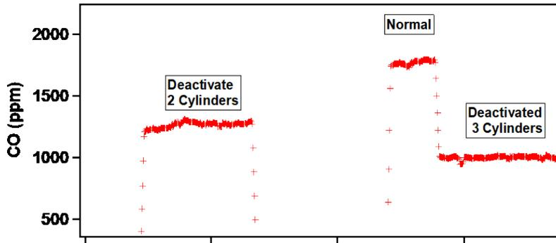
(ECM). A previous study shows deactivating engine cylinders at low engine loads (<15%) increased combustion efficiency and reduced methane emissions by 56%-60%. Similarly, the concentration of CO, another incomplete combustion product, is reduced by 30% and 44% respectively when two and three cylinders are deactivated, as shown in Figure 18. While no
