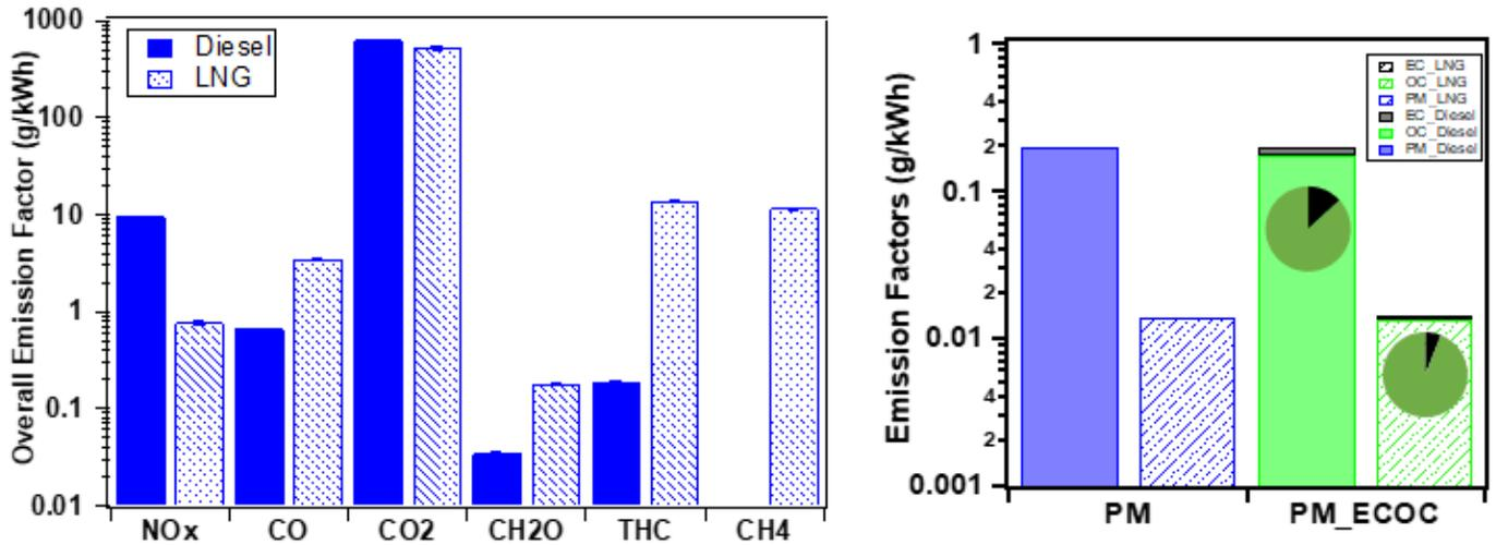
**FIGURE 15 OVERALL EMISSION FACTORS FROM A DUAL-FUEL ENGINE**
