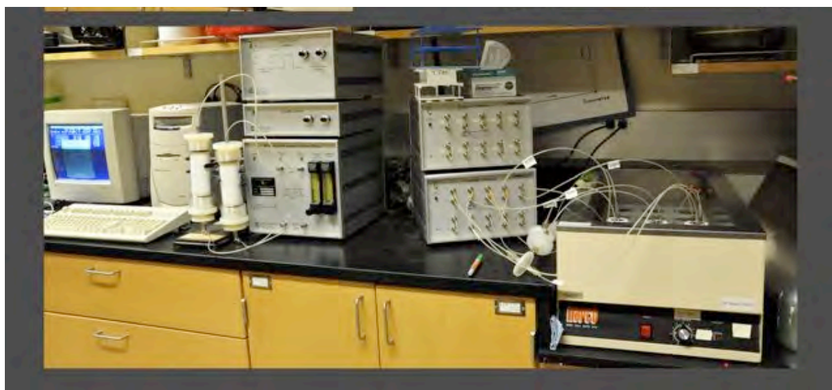
Figure II-D-1: Respirometer equipment used for aerobic biodegradation monitoring in 29-day tests.
