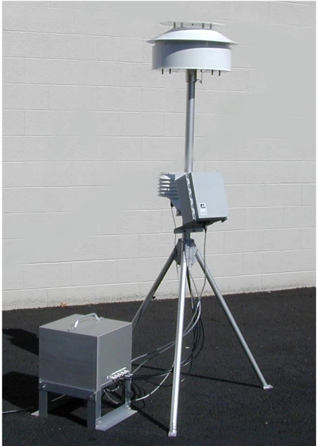
Figure AT.1: Photo of SASS monitor including vacuum pump box
