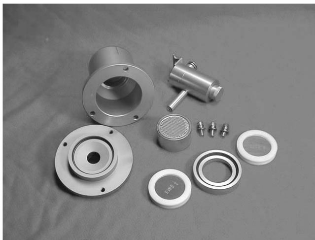
Figure AT.2: Disassembled SASS canister, including sharp cut cyclone
