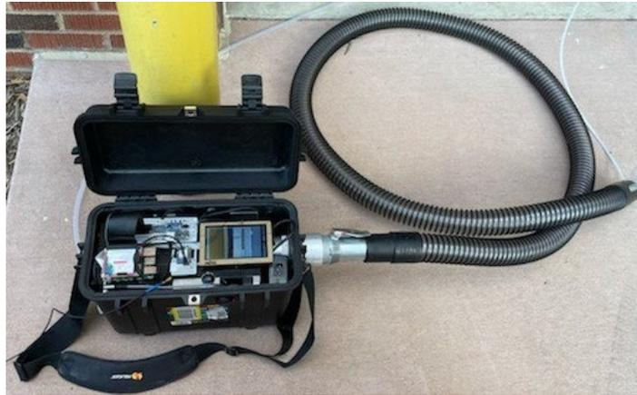
Figure 2: Integrated OS-HFS instrument during initial Testing.
