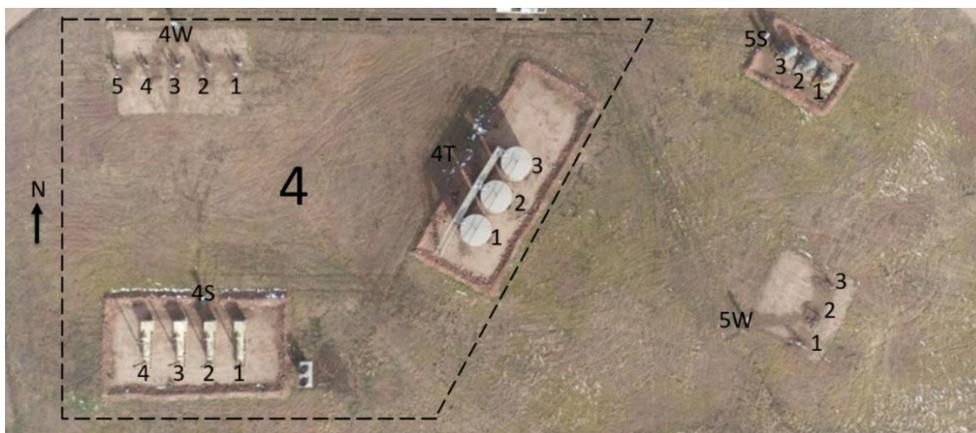
Figure 43: Pad 4 at METEC with equipment groups marked.
