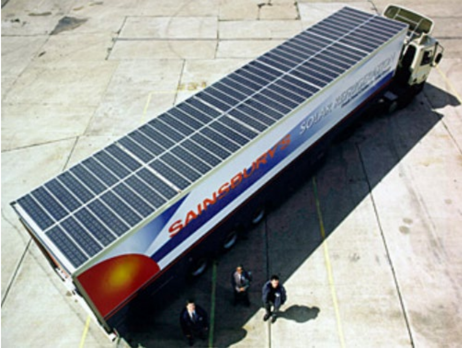
Figure 31: Trailer with Solar Assist 192
