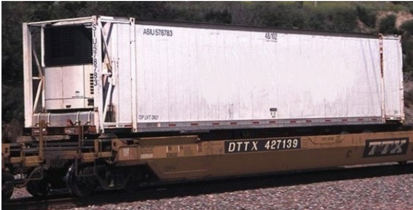
Figure 2: Domestic Shipping Container TRU
