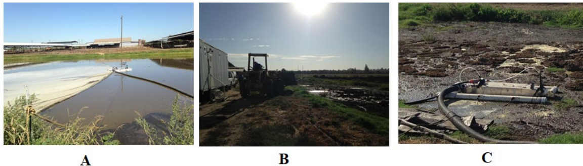
Figure 21. (A) The wind tunnel floating on the lagoon; (B) removing the scum layer from the surface of the settling basin; and (C) floating the wind tunnel on the settling basin at the Foxtrot dairy.
