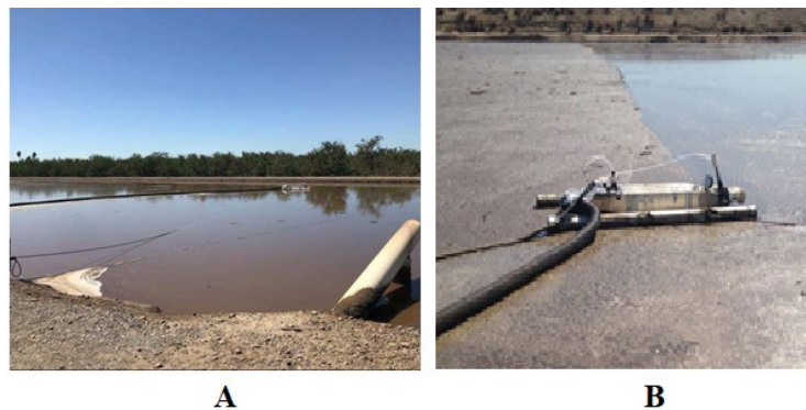
Figure 17. (A) The wind tunnel on the lagoon; and (B) the wind tunnel on the settling basin at the Delta dairy.
