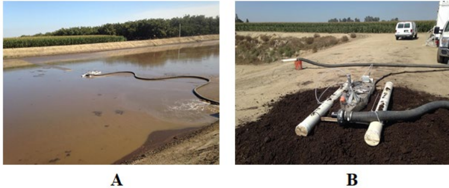
Figure 16. (A) The wind tunnel on the lagoon; and (B) the wind tunnel over manure collected from the compost-bedded pack barn at Charlie dairy.
