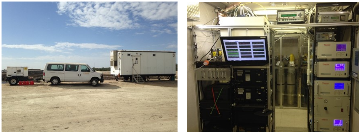
Figure 10. (A) The Mobile Air Quality Laboratory (MAQ Lab) and engine-generator set; (B) different analyzers and supporting equipment onboard of the MAQ Lab.
