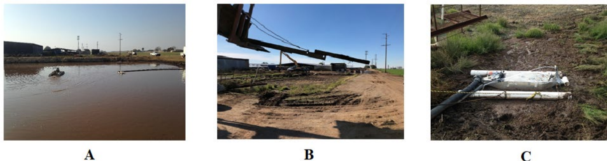
Figure 14. (A) The wind tunnel floating on the lagoon; (B) removing the scum layer from the surface of the settling basin; and (C) floating the wind tunnel on the settling basin at the Bravo dairy.
