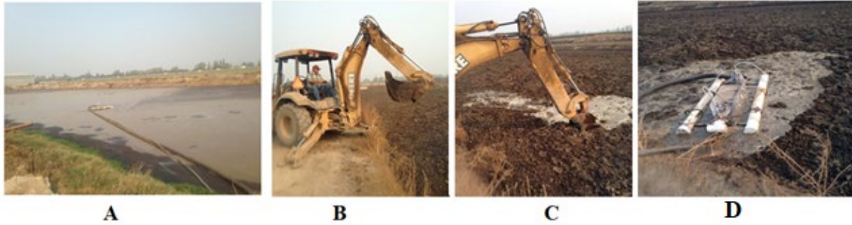
Figure 12. (A) The wind tunnel floating on the lagoon; (B and C) removing the scum layer from the surface of the settling basin; and (D) floating the wind tunnel on the settling basin at the Alpha dairy.
