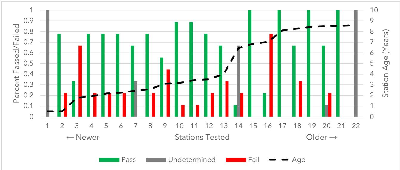
Figure 9: Fueling performance test results for each station.
