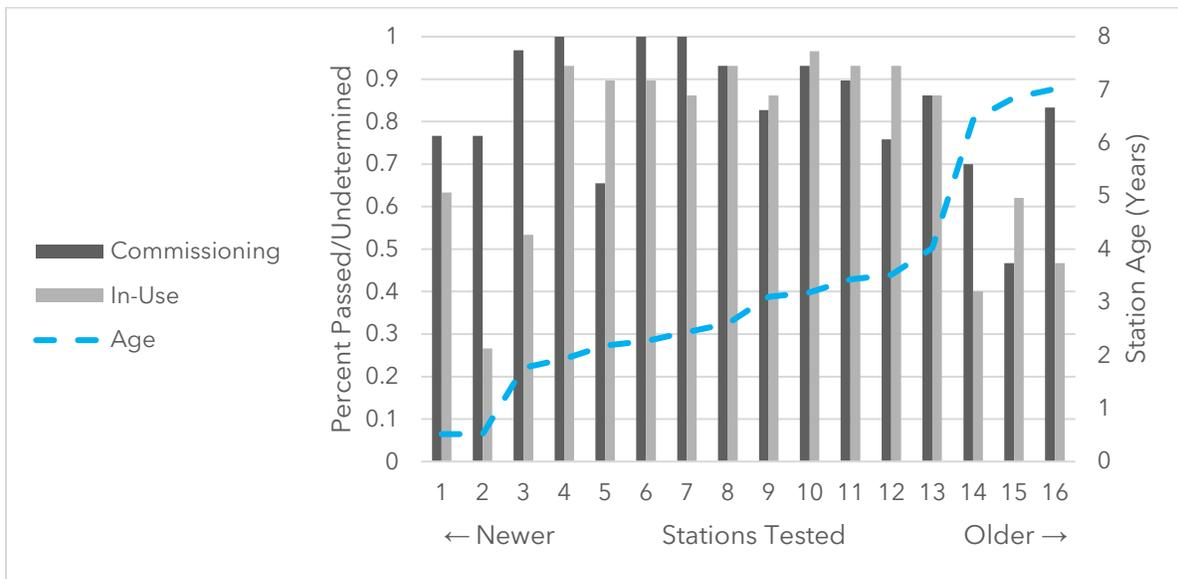
Figure 14: Station passing rate during commissioning and in-use testing by station age.
