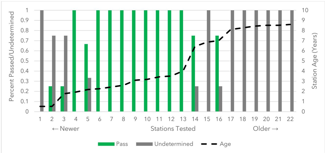
Figure 6: Protocol fault test results for each station.
