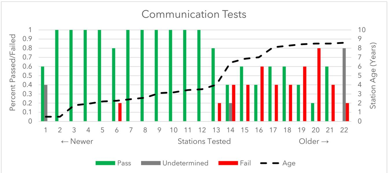
Figure 8: Communication test results for each station.
