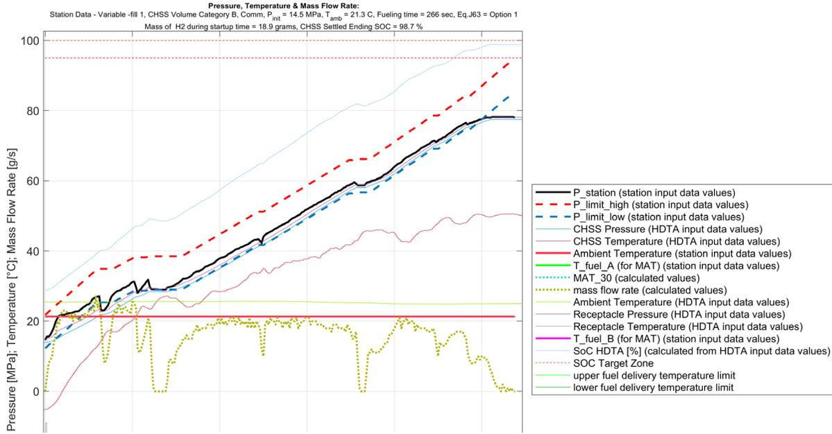
Figure 12: Example of fill ending with lower pressure corridor tolerance fault above 95% SOC.
