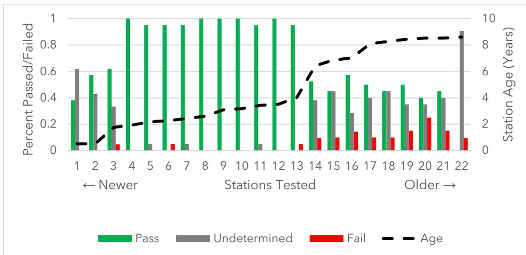
Figure 5: General fault and communication test results for each station.
