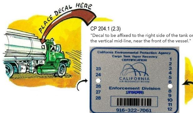
2. **Cargo Tank Number.** The CARB-issued Cargo Tank Number for the vessel should be displayed on the cargo tank in a location that can be visible. (CP 204.1 (2.3)). The preferred location is on the left side of the tank, either stamped on the first tank mount or as a vinyl numerical decal on the vertical mid-line near the front.
