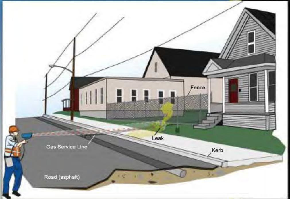
deduce the relative methane concentration. This signal is processed so that methane concentrations can be reported in parts per million meter or ppm-m. The laser has a maximum distance of up to 100 feet and is selective to methane only. It will not false alarm on other hydrocarbons.
