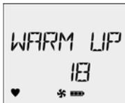
The LCD displays a countdown of the time remaining (in seconds) for the pump to warm up.
