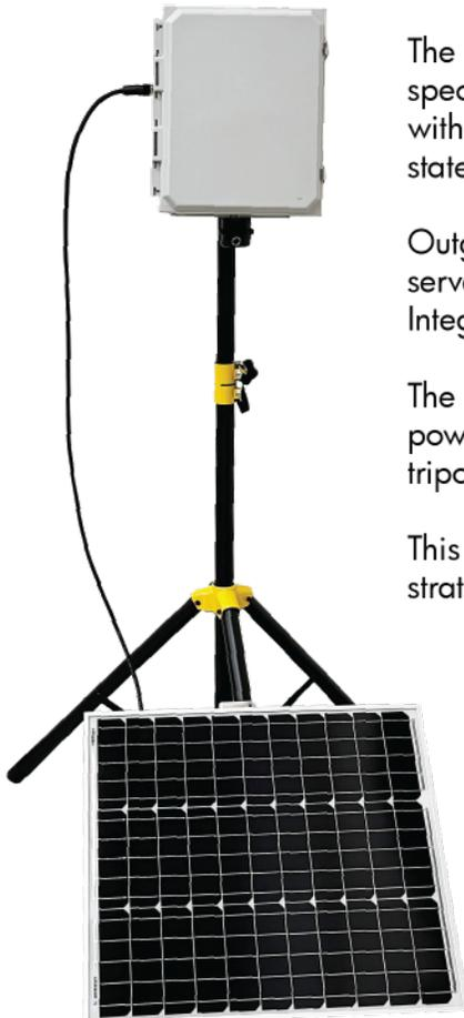
The **GAS•TRAC<sup>®</sup> FMD** is an active sampling system equipped with a tunable diode laser spectroscopy (TDLAS) cell capable of detecting methane as low as 200 PPB. When equipped with an anemometer, the **FMD** is capable of localizing leaks, as well as providing state-of-the-art data to aid in quantification.
