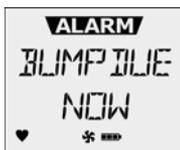
If **Force Bump** is enabled, enter a value (1-365) in the **Bump Interval (days)** field located in the **Sensor Configuration** section.
