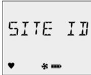
To enter a number from **1-999**, continue pressing  until the desired number displays. To scroll rapidly, press  and hold.
