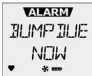
Apply gas while **BUMP DUE NOW** displays. Verify the visual, audible, and vibrator alarms activate. The detector must enter alarm to pass the bump test. For complete instructions, refer to [Bump Test](#).
