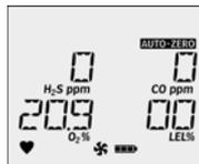
If the **Force Calibration** option is enabled and the sensor(s) is past due for calibration, the sensor will not auto zero during startup. The sensor must be calibrated.
