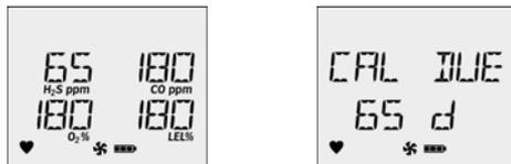
If a sensor fails to span successfully and it is past the calibration due date, the following screens display.
