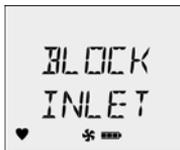
Using your finger, block the end of the hose. The following screen displays.
