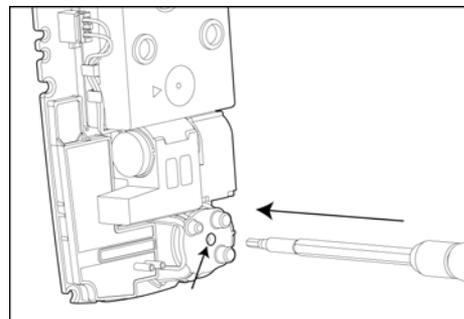
**Figure 11. Remove the O<sub>2</sub> Sensor With a Screwdriver**
