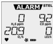
Enter the interval (**5-15 minutes**) in the **STEL Interval (minutes)** field. The detector is shipped with the STEL interval set to 15 minutes.
