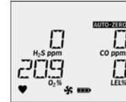
When auto zero is complete, the detector beeps two times.
