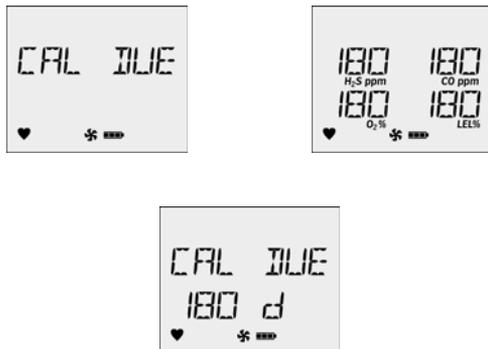
The number of days that displays in the **CAL DUE XXX DAYS** screen is the earliest date (overall of all sensors) a calibration must be performed.
