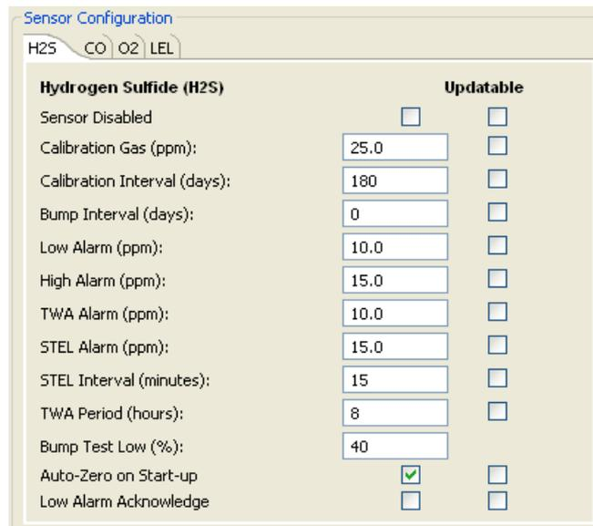
**Figure 5. Sensor Configuration Tab (H<sub>2</sub>S)**
