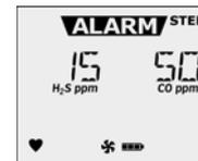
3. After entering the STEL setpoint, the STEL interval value (**5-15 minutes**) must be entered. Refer to [STEL Interval](#).
