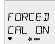
Press  to acknowledge. Refer to [Calibration Procedure](#) to begin calibration. If  is not pressed to enter calibration within 2 minutes, the detector automatically deactivates.
