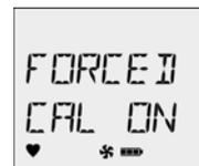
The sensor(s) must be calibrated to continue and enter normal operation. For complete instructions, refer to [Calibration](#).
