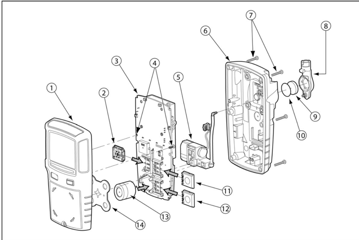
Figure 9. Replacing a Sensor or Sensor Filter
