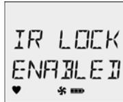
If **IR LOCK ENABLED** is enabled, the sensor(s) must be calibrated using the IR Link or the MicroDock II station. For more information, refer to [Cal IR Lock](#) in User Options.
