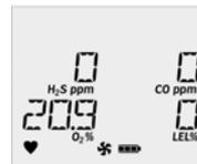
The detector begins recording the maximum gas exposure (MAX), and calculating the short-term exposure level (STEL) and time-weighted average (TWA) exposures.
