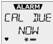
Press  to acknowledge the warning. If  is not pressed within 2 minutes, the detector automatically deactivates.
