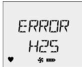
In auto span, an error message displays if the target gas does not meet the expected values.
