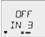
The detector then reactivates and performs the calibration countdown. Continue to hold
