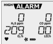
During a pump alarm, **HIGH** and **ALARM** display, and
