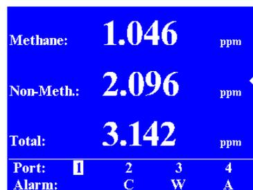
The 9000 Methane/Non-Methane analyzer uses a flame ionization detector (FID) in conjunction with an oxidation catalyst that oxidizes all hydrocarbons except methane to produce a methane measurement which is then subtracted from the total concentration to determine the non-methane hydrocarbon reading.
