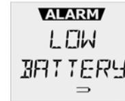
The low battery alarm continues 10 minutes. If the battery voltage drops too low, the detector activates the automatic deactivation alarm.
