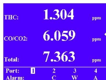
The 9000 Total Carbon analyzer utilizes a flame ionization detector (FID) in conjunction with a catalytic methanizer that converts the CO and CO<sub>2</sub> to methane (CH<sub>4</sub>) and leaves the hydrocarbons unchanged for a total carbon measurement which is then subtracted from the total carbon concentration to determine the combined CO/CO<sub>2</sub> reading.
