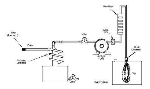
Figure 3-2 – Integrated Gas Sampling Train
