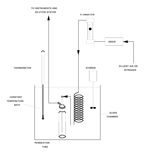
Figure 15-3. Apparatus for Field Calibration
