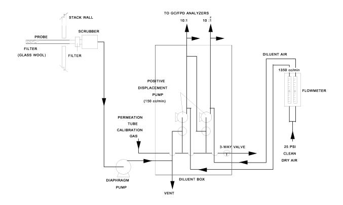
Figure 15-1. Sampling and Dilution Apparatus
