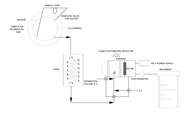
Figure 15-2. Gas Chromatographic Flame Photometric Analyzer
