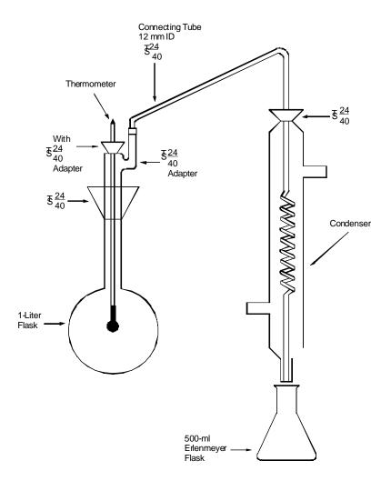
Figure 13A-2. Fluoride Distillation Apparatus.
